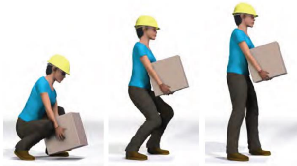
Figure 28: Lifting the load
