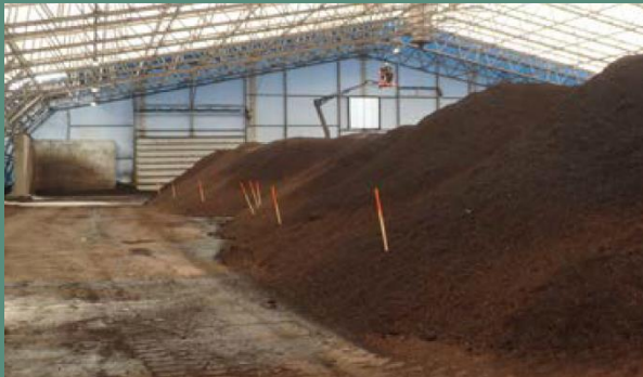
Figure 260: Identification of piles (wooden stakes)
